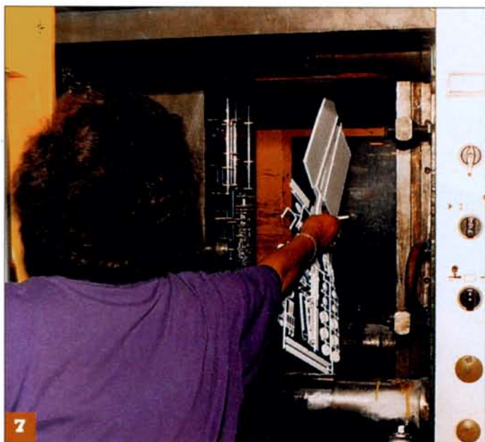
Once it's cooled enough to touch, the mold releases the model and it can be pulled from the machine.
