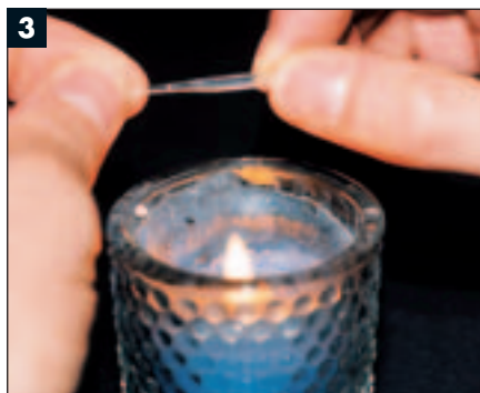
3 To make the miniature bottle of hot sauce, David began by stretching a piece of clear sprue.
