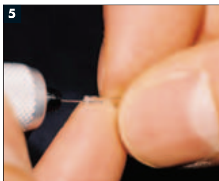
5 Tight work: drilling out the inside of the bottle with a pin vise.
