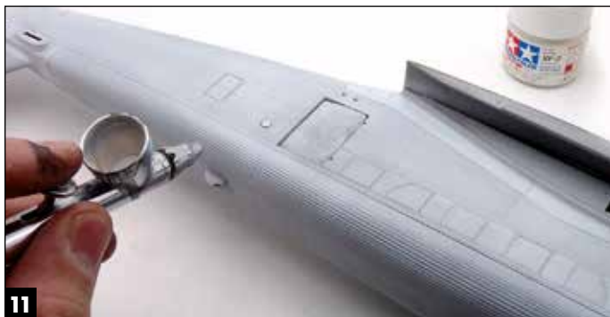
11 To intensify the red to come, I airbrushed flat white (XF-2) as a base coat.
