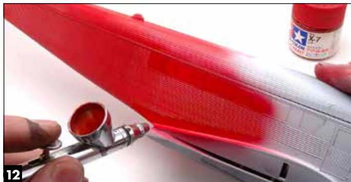
12 Brightened by the white, the red acrylic (X-7) seems to vibrate.
