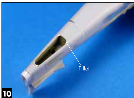
10 After breaking off one of the tail-wheel doors, Rato thought it would be a good idea to replace both of them with scratchbuilt ones. He started by correcting the shape of the tail-wheel well.
