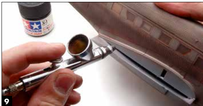
9 To lend depth to the skin without exaggerating the effect like a wash might, I airbrushed a dilute mix of Tamiya acrylic black (X-1) and alcohol.
