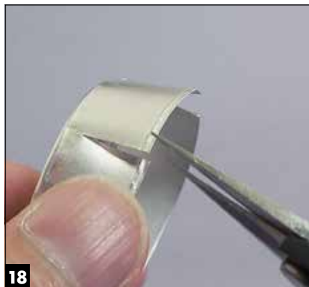
18 Foil from a votive candleholder provided easily malleable material for the wing's twisted panels. Waikong cut it with Xuron scissors made for photoetched metal.
