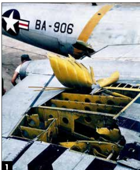
Photos taken immediately after the mission show a gaping hole in the starboard wing, additional damage in the flap area, and the fuselage shot that disrupted electrical power and wounded Capt. Joyner.
