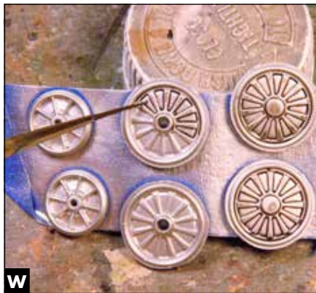
W A sealing coat of PFM helps washes flow into engraved detail. John painted the areas between the spokes black.
