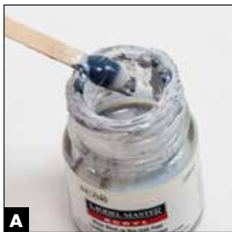
A Paint performs best when the components are mixed. A sludge of settled pigment and filler covers the bottom of this bottle of paint.
