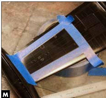
M Low-tack tape sticks to curved and uneven surfaces better than Post-it notes when masking panels.
