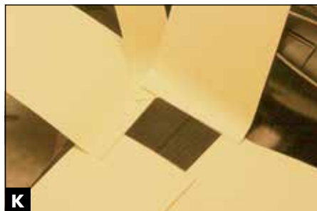
K Post-it notes have straight edges and low-tack adhesive — ideal for masking panels.
