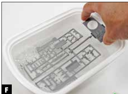
F Washing the sprues in a tub eliminates the chance of losing a part down the kitchen drain.
