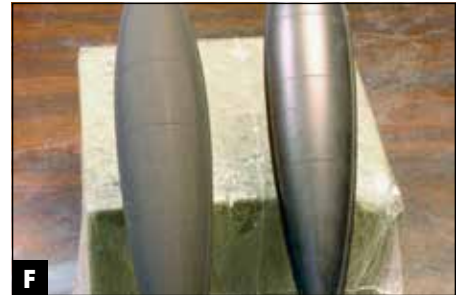
F Smoothing corners and details, such as ridges on the drop tanks, is just as important as tending big surfaces. A tack cloth removes sanding dust.
