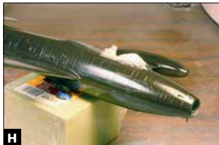
H It takes time, but after multiple coats of PFM, with sanding in between, John's F-84 had a glass-smooth foundation for the metallic finish.
