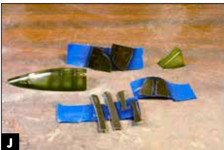
J John painted and glossed the gear doors and canopy at the same time as the airframe to ensure they had the same sheen.
