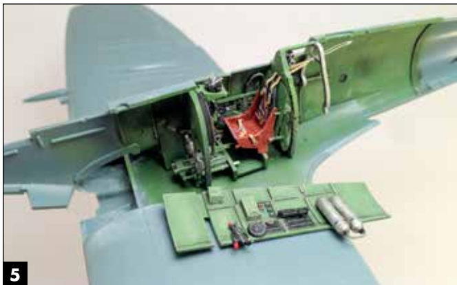
5 Careful test-fitting ensured the cockpit and wings would fit, not fight.
