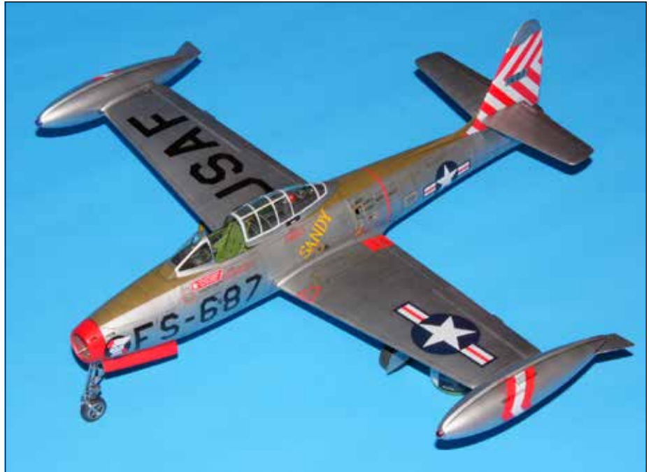
Layers of clear acrylic and Alclad II lacquers give John's 1/32 scale F-84 a sturdy natural-metal finish.
