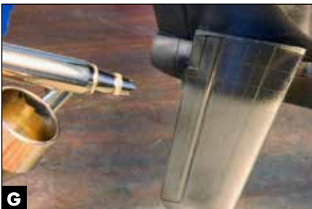
G Here comes the shine: In this case, light coats of PFM are applied straight out of the bottle a section at a time.
