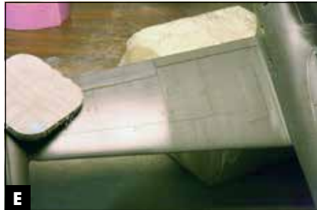
E John discovered flat paint is easier to smooth than gloss paint is to apply. The outboard section of the F-84's wing has been sanded.
