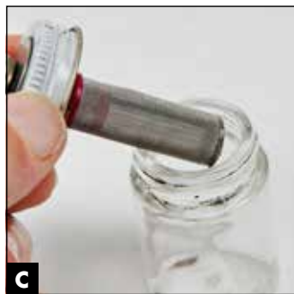
C This simple filter prevents paint blobs or chunks from clogging the airbrush or marring your model.
