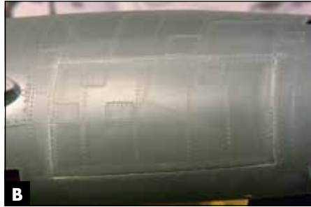
B Careful sanding removed the shine left by the glue. Thin and unforgiving, metallic paints reveal even small differences in surfaces.
