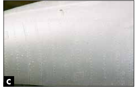
C Sanding generates not only dust but also static electricity, which attracts more dust and fluff — schkootz , the bane of natural-metal finishes.
