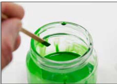
The flow test is a good measure of getting the right consistency for airbrushing. If a drop of paint runs down the side of the mixing jar smoothly and leaves an even film it's ready (left). If it doesn't run, it's too thick (center), and if runs fast and leaves an uneven film of color, it's too thin.
