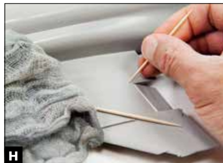
H Dust is the enemy of good paint. A toothpick gets it out of panel lines; a tack cloth takes care of the last bits before airbrushing.
