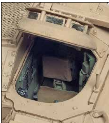
All of the hatches open to reveal the Bradley's interior. This is the driver's position.
