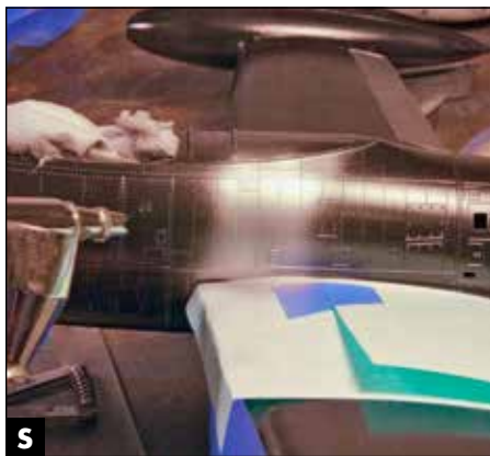
S Paint swirling around in corners can dry prematurely, creating grit. To prevent this, John masked surrounding surfaces not being painted.
