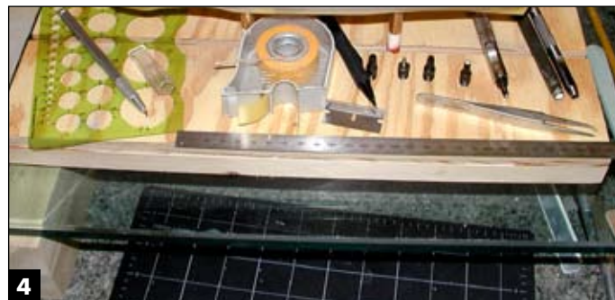
4 To mask the deck, Ron applies small, overlapping pieces of tape. His tools are a circle template, stencil knife, Tamiya tape, toothpick, .5mm technical pencil, razor blade, punches, tweezers, straightedge, and a cutting mat.
