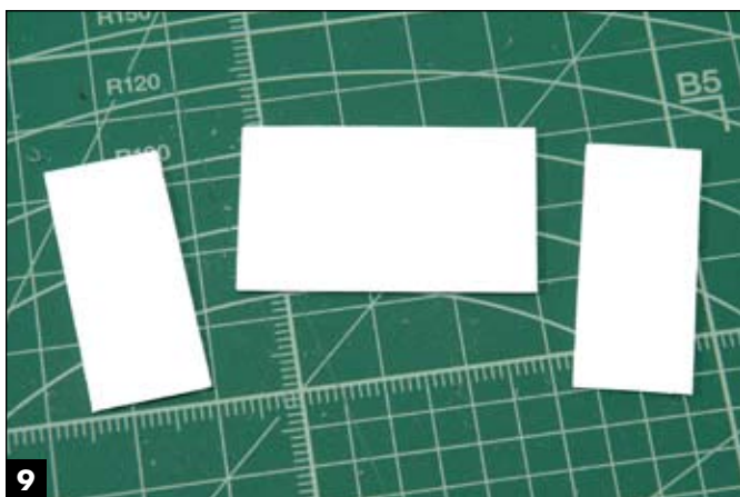
The Humvee's armored back wall consists of two 14mm x 33mm seat backs and a 36mm x 22mm center panel cut from .030" sheet styrene.
