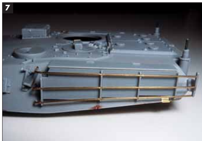
The kit-supplied plastic stowage rack bars were replaced with brass wire. Also note the tow cable mounting sleeve, made from sheet brass.
