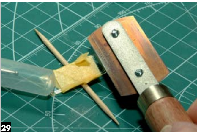
... then removes a small sliver of the body of the window on the opposite end, restoring the ledge.
