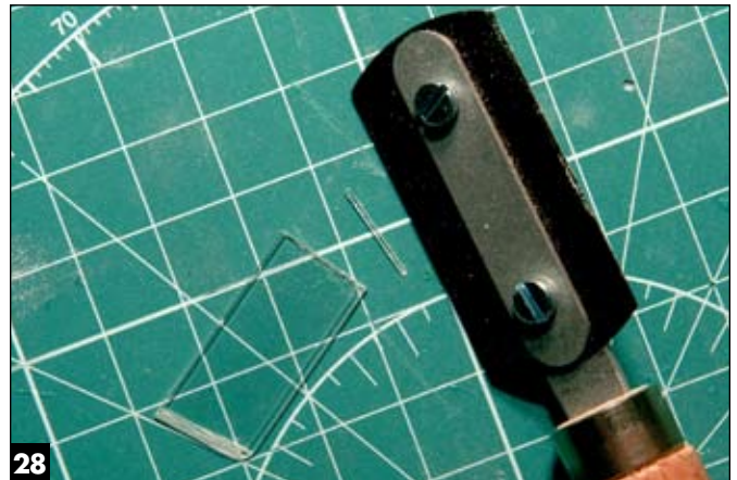
Armoring the windshield glass, Aaron sands the locating ledge from the vertical edge of a kit windshield piece ...
