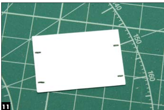
The center panel features mounting holes on each side made with a drill bit and opened with a knife.
