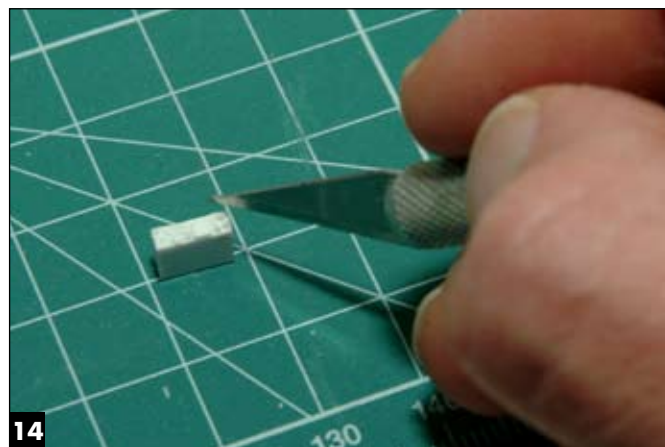
Salami-sliced styrene rod of differing diameters provide dials and sockets for the front of the radio unit.
