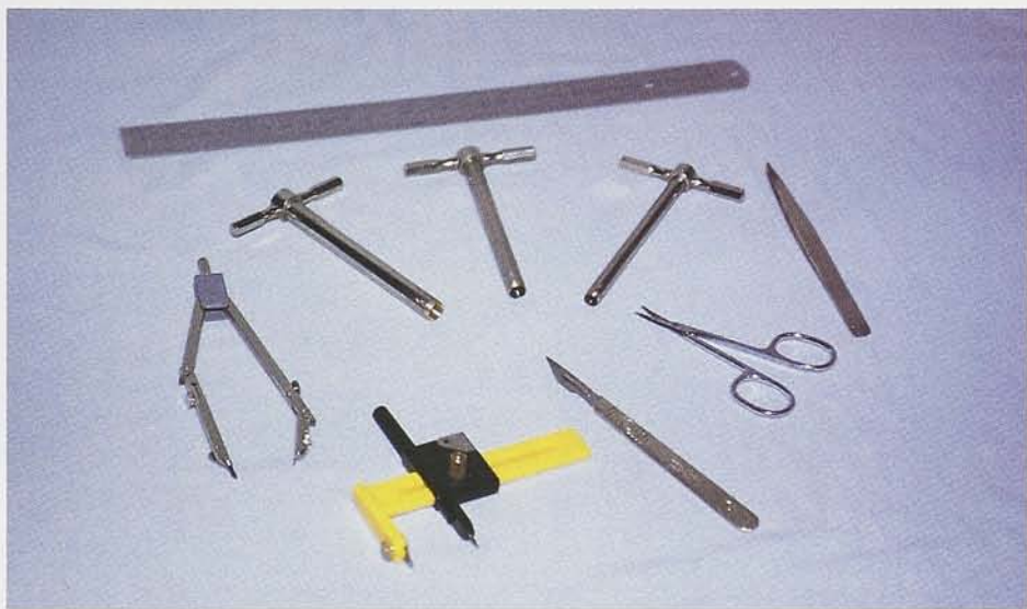
Fig. 2. T-handled punches, a compass cutter, and cuticle scissors are needed to cut the colored discs from solid-color trim decal. ▶
