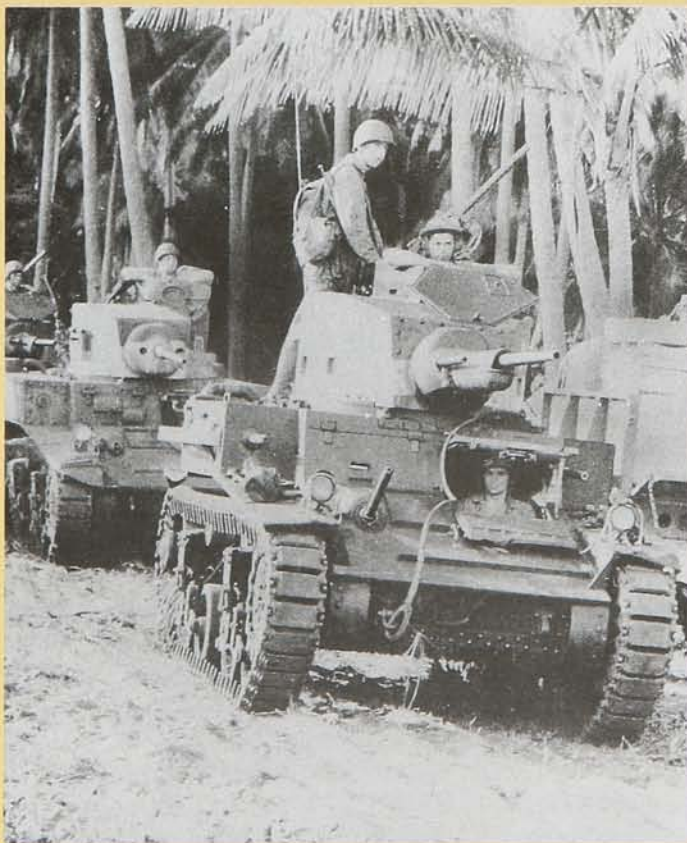
An M2A4, followed by an M3, skirts the jungle's edge on Guadalcanal in 1942. Photo courtesy of R.P. Hunnicutt.
