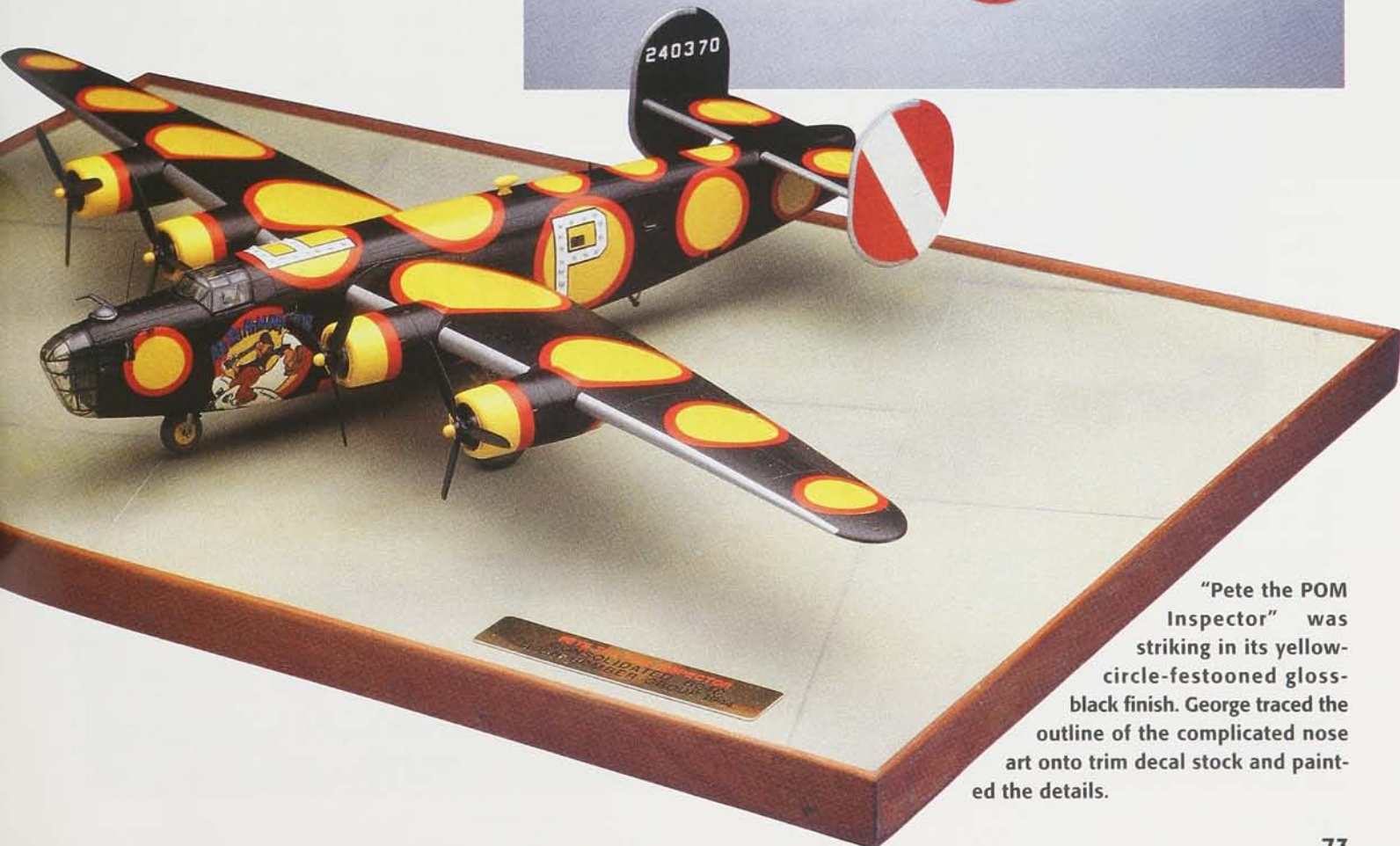
Fig. 5. The yellow discs under the inboard engine nacelles had to be made in two pieces to fit the compound curves. ▶
