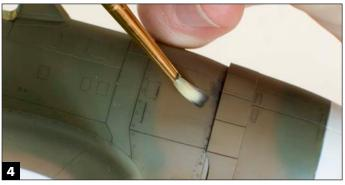
Next, with a wider brush, I pull the pastel back in the direction of the slipstream. If you don't like the effect of the pastel, you can remove it with a damp cotton swab, and when the area is dry, you can have another go. I examine the model and look for indentations (like around the turbocharger vents) and use the pastel to force shadows into those corners.
