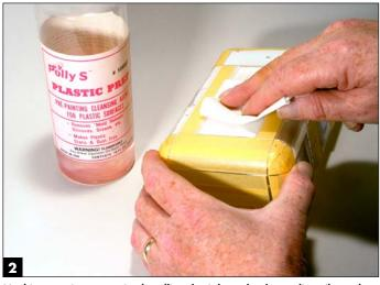
Masking requires extensive handling that's bound to leave dirt, oils, and adhesive residue. Polly S Plastic Prep cleans up for better paint adhesion.
