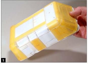
Mark masked the entire exterior of the clear piece, then used a hobby knife to trim away and expose the frame and areas that would receive paint.
