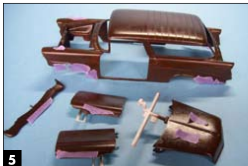
5 Strips of tape mask the rustiest areas, such as the tops of doors, center of the hood, and the corroded wheel arches.
