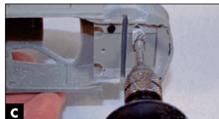
C Using a motor tool, Wayne removes pour plugs from the body of the car so the interior and chassis will join cleanly.
