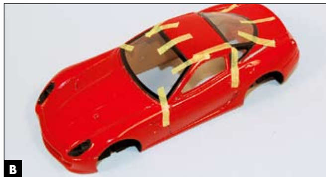
B To ensure a solid fit, Wayne held the clear pieces in place with strips of Tamiya tape for 24 hours.
