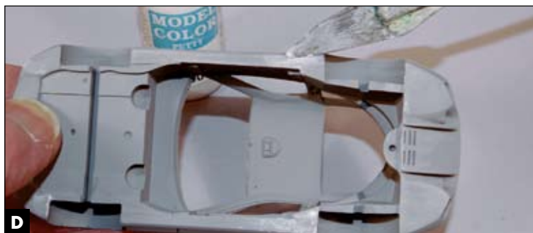
A Wayne removes ragged edges left by the casting process from the windows with an emery board he trimmed to a point.
