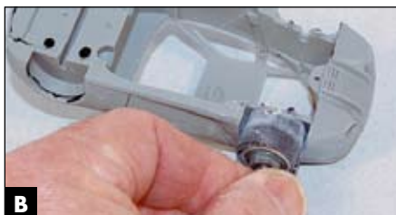
B Hand-spun modeling: A motor tool sanding wheel wrapped with wet/dry sandpaper is the perfect fit for the Ferrari's wheel arches.
