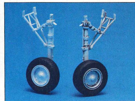
8 Compare the bland, sterile main landing gear on the left to the “sludge washed” unit.
