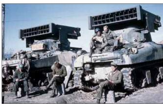
Even when fitted with M17 rocket launchers, these Shermans could also be used as chairs during mail call. Note the differences between the welded (left) and cast hulls. U.S. Army photo
