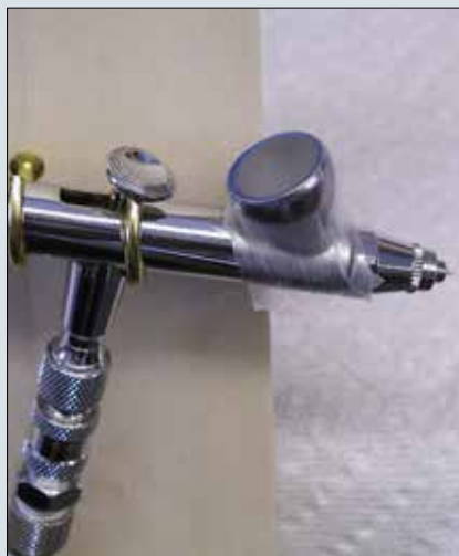
Parafilm M is a great way to cover an airbrush cup to prevent sloshes and spills.
