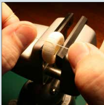
James uses heavy cotton thread to put tread pattern back on a resin tire. The pattern was lost through gluing, filling, and sanding.
