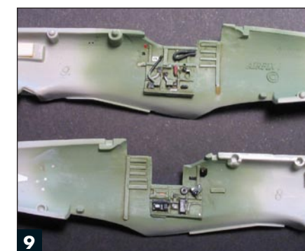
9 The Hi-Tech set included sidewall inserts. Rato thinned inside the fuselage to make room, installing the sidewalls after painting and detailing.
