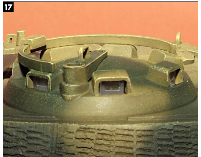
17 Backyard Armor also supplied the clear-resin periscopes for the commander's cupola and other periscope openings on the hull.
