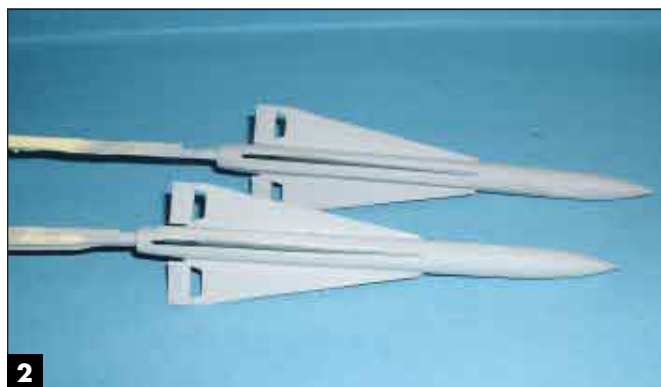
2 Mounting the missiles on rods made them easier to handle during painting.
