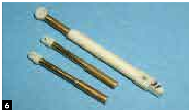
6 Michael added brass tubing to the launcher's hydraulic arms to change the angle of the launcher platform.
