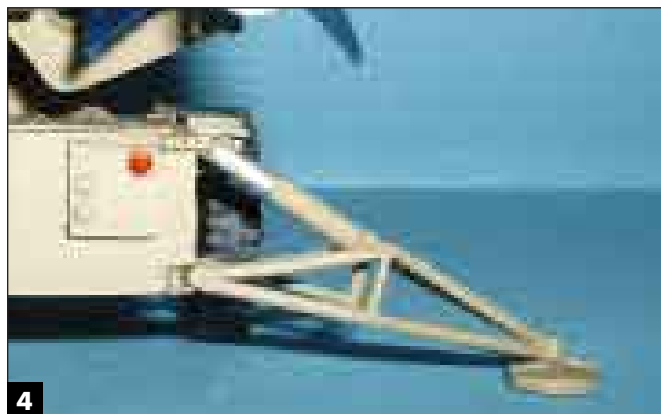
4 Lengths of brass tubing strengthened the model's delicate legs.
