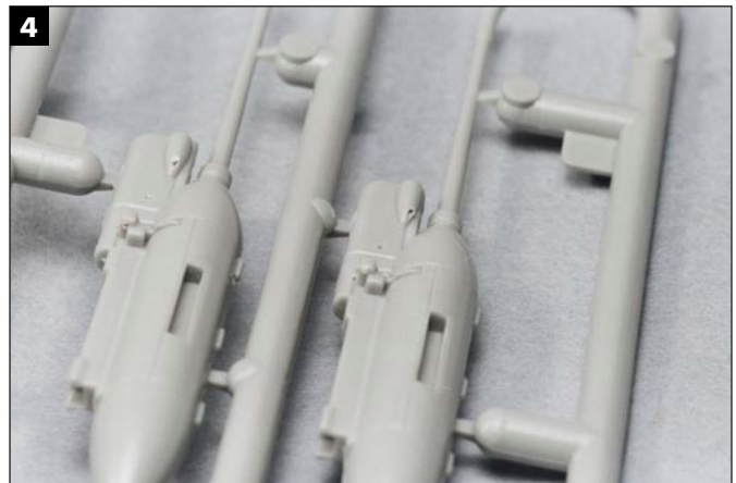
4 The cannons are prepared for plumbing by drilling in four locations with a #80 drill.
