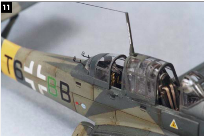
11 A view of the MG81Z breech, ammo belts and sights; also note the open canopies and the mast stencil.
