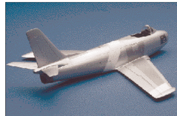
11 Note the smoothly faired aft fuselage section typical of A-model Sabres.
