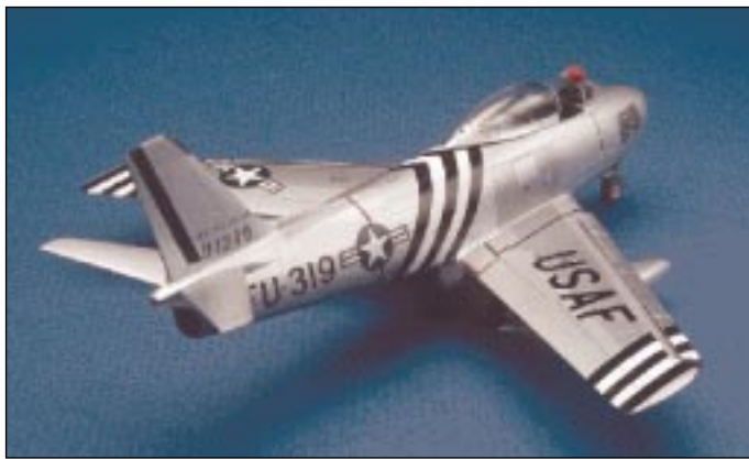
Early Sabres had automatic leading-edge slats on narrow-chord wings. The horizontal stabilizers were conventional (not "all-flying" as in later models).
