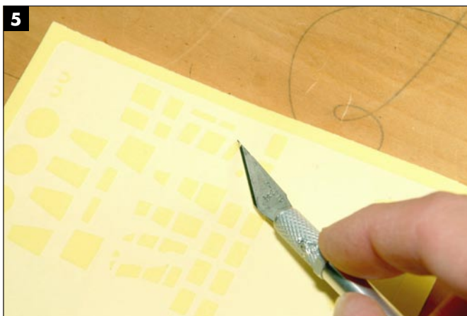
5 Aaron uses a sharp hobby knife to begin peeling the corner of a mask from the backing sheet. Once started, he held the mask between his thumb and the blade to pull it away entirely and transfer it to the model.
