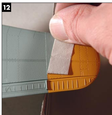
12 Aaron removes a mask, folding the tape back on itself and working slowly to avoid damaging the paint underneath.
