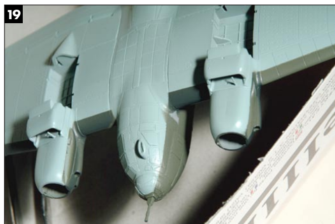
19 Paint lifted off the model around the wing fuselage root when the masks were removed.
