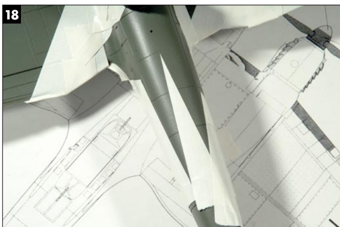
18 Using scissors, Aaron cut the sharp points and odd angles necessary for the Luftwaffe splinter-scheme camouflage.
