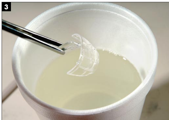
Aaron dipped clear parts in Future floor polish, dragging each across a paper towel to wick away excess liquid before setting it aside to dry.
