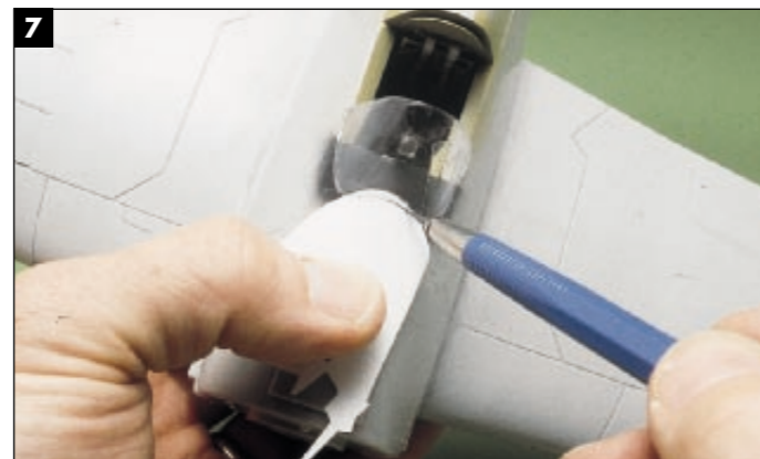
The gap in front is too large for super glue, so it must be filled with sheet styrene.
