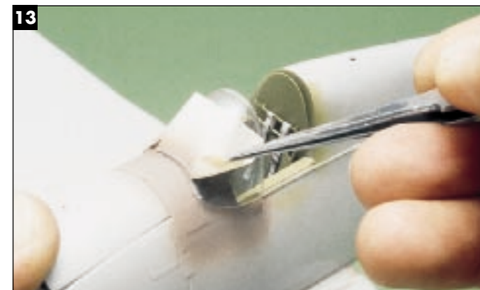
After a primer coat, Pat removes the mask to check the joint.
