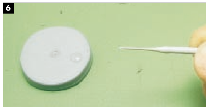
Biting the end of stretched styrene sprue produces a handy super glue applicator.
