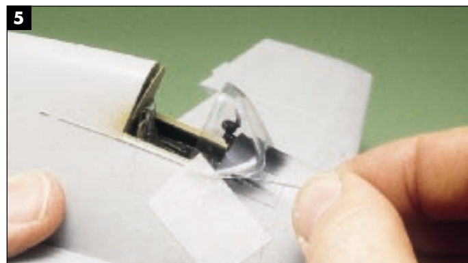
Tiny drops of super glue won't frost the clear parts.
