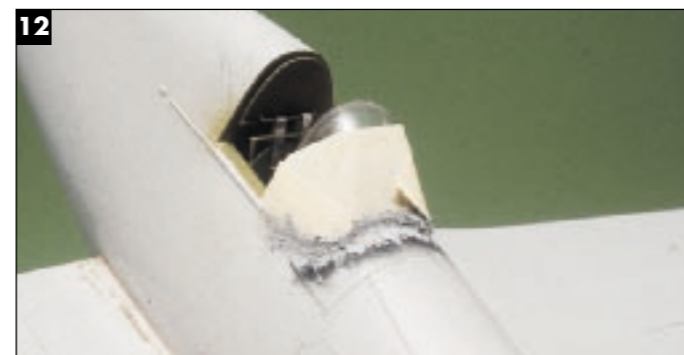
With the clear windows masked, Pat fills any remaining gaps with filler putty.
