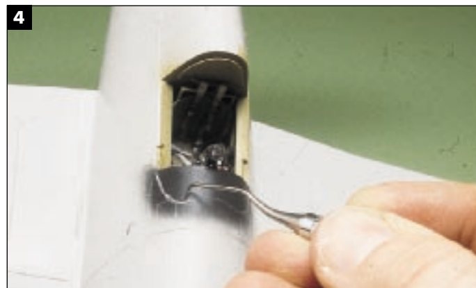
Scraping away paint improves the glue's adhesion.
