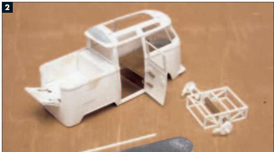
Roger bent the passenger compartment floorboard from .030" brass sheet, removed the side door, cut out the tailgate, and cut a rectangular hole in the top for the sunroof. A sheet styrene divider separates the passenger cab from the pickup bed. He made the front suspension subframe from square styrene rod and modified the front axle by replacing its center section with a brass rod.
