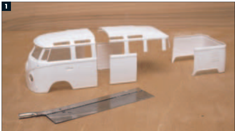
Roger started by sawing the body at the appropriate places. The van body was shortened, glued back together, then cut apart lengthwise to be narrowed.
