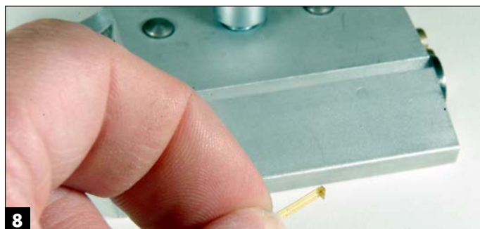
8 For smaller parts such as fender brackets, Aaron uses 3Detail's bender. It's small, easy to handle, and produces a perfect right-angle bend every time.
