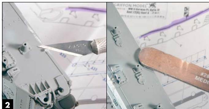
2 (Left) After assembling most of the lower hull, Aaron carves off a ridge at the top of the hull molded to represent a fender bracket. (Right) A sanding stick removes the remaining plastic and leaves the part flat.
