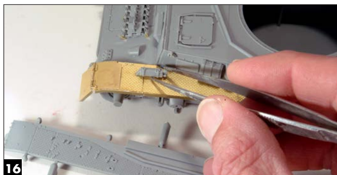
16 The brass fenders didn't have locating holes for the tools. Aaron used the kit's plastic part as a key to place items such as the fire extinguisher on the front left fender.
