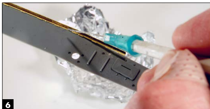
6 Attaching the parts is easy: Aaron holds the fender bracket in place and uses a needle point to deliver a bit of liquid super glue to the gap, allowing capillary action to draw it along the join. He uses accelerator to set the glue, then adds a little more glue to bolster the bond.
