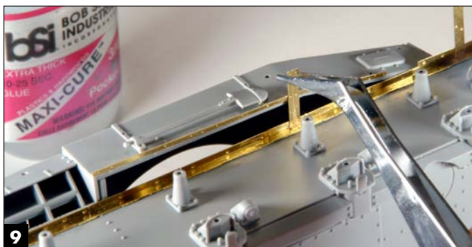
9 Tweezers and super-glue gel make quick work of attaching the fender brackets. Griffon marked attachment points clearly, so the job was easy. The slower-setting gel allowed time to align the part.
