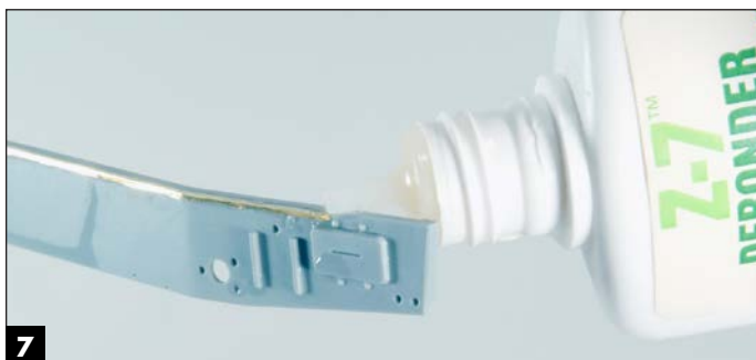
7 Unfortunately, after attaching the bracket Aaron discovered that it needed to extend past the edge of the plastic part. A little debonder saved the day, as a drop on the joint enabled him to pop the part loose.
