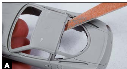
A Wayne removes ragged edges left by the casting process from the windows with an emery board he trimmed to a point.
