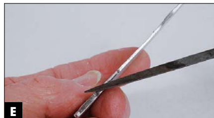
E Although the white-metal parts are nearly perfect, Wayne uses files to remove mold lines from items such as the exhaust pipes.
