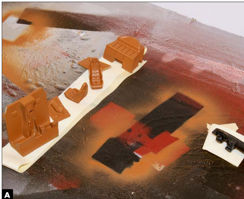
A Wayne taped the interior parts to cardboard, then airbrushed them leather. He painted the inside of the body shell flat black at the same stage.
