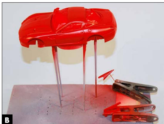
B Attaching the body to a homemade spray stand allows Wayne to turn the model around to get paint into every nook and cranny.
