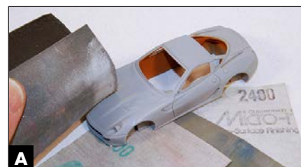
A A smooth primer surface yields a good finish. Wayne block-sands the primed body with 2400- and 3200-grit polishing cloths.
