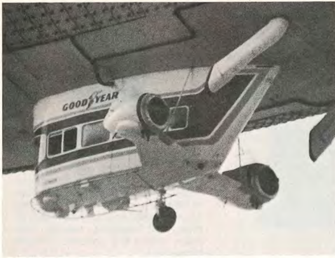
Fig. 4. Close-up of Columbia's gondola. Note the footrails, pylon support struts, and exhaust pipes projecting through the cowlings.
