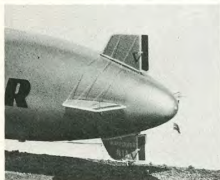
Fig. 6. Stretched sprue was used for the support wires on the fins, control cables, control horns, and the flag line.
