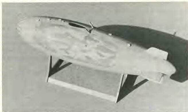
Fig. 1. The rectangular hole for the illuminated sign has been backed with sheet styrene, filled, and smoothed with sandpaper.
