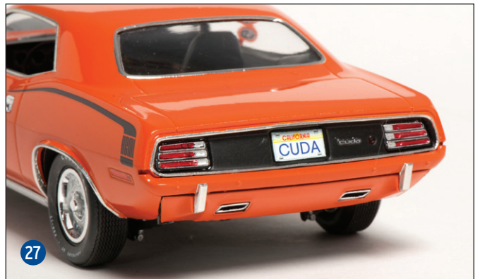
27 Body color elastomeric rear bumpers were a midyear addition in eight colors (other than Rallye Red), and thus are rarely seen on 1:1 1970 'cudas. The rear exhausts should extend a little farther beyond the roll pan than shown here; I'll correct that on my next build of this kit.
