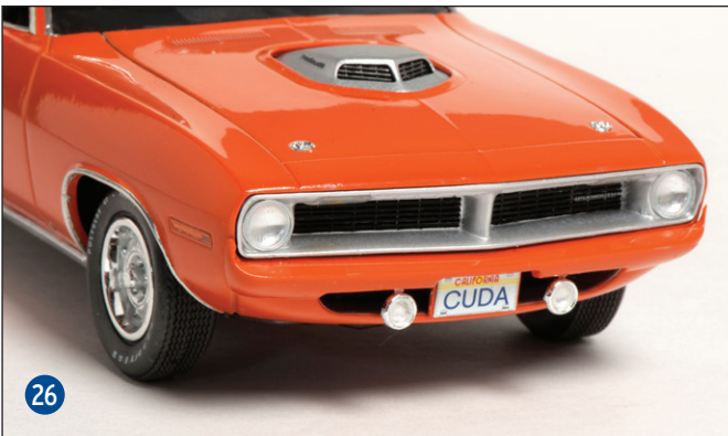
26 Revell includes the Elastomeric front bumper as a build option, and exactly like its 1:1 scale counterpart, this bumper is shaped differently than the plated front bumper. Those fog lamps are correct in appearance, but contain delicate mounts; you may want to reinforce them with pins.
