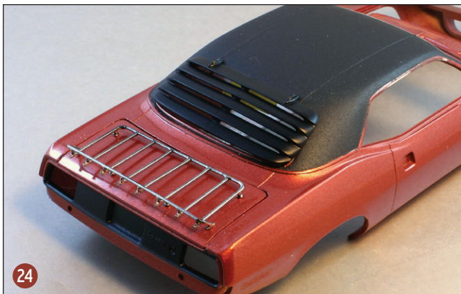
24 The completed trunk rack was sprayed gloss black, then airbrushed with Alclad chrome. I was pleased with the final product, but I'm sure one made from metal would be even more convincing.
