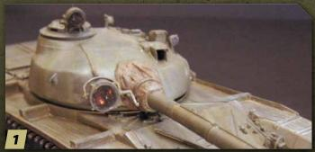
Tank anatomy lesson! The mantlet is an armored shield that protects the opening where the gun's barrel attaches to the turret. Many mantlets wear a canvas cover or tarp wrapped around them. Such is the case on this T-72 main battle tank.
