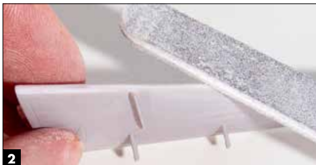
The primer also revealed that Aaron hadn't been thorough when he sanded the leading edge of one wing. When the primer line disappears, the gap is smooth.
