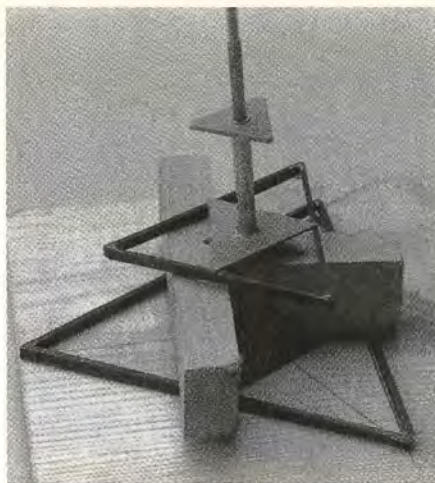
Fig. 1. Simple jig: Wood scraps hold Plastruct structural forms in place during construction of the mooring mast.
