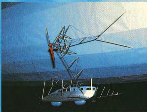
The rear gondola powered a propeller at the rear and two outriggers on the side of the envelope.
