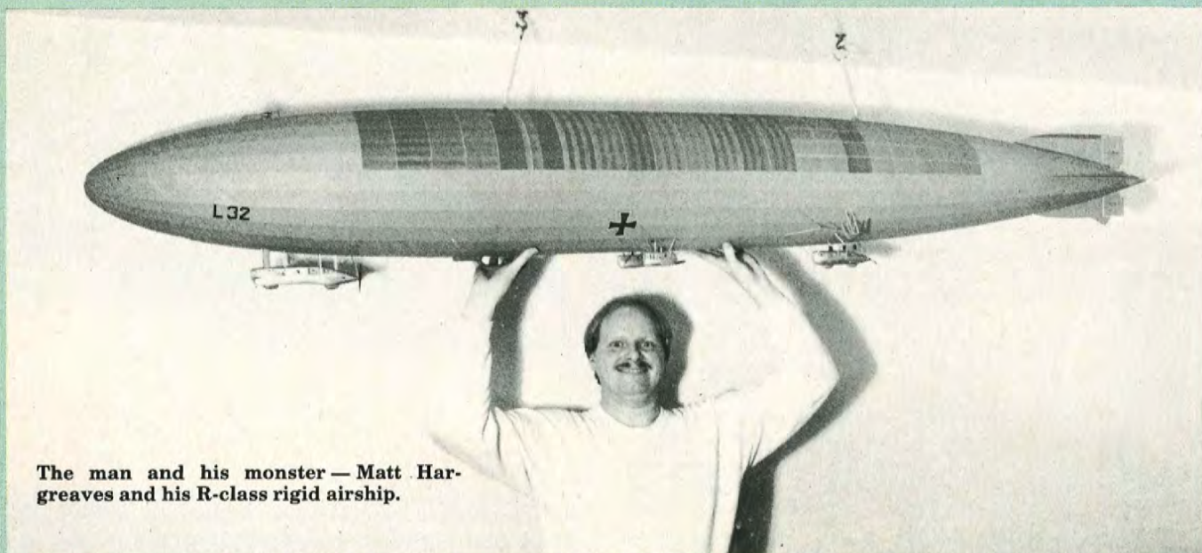
The fins were fashioned from Plexiglas and inserted in slots in the envelope formers.
