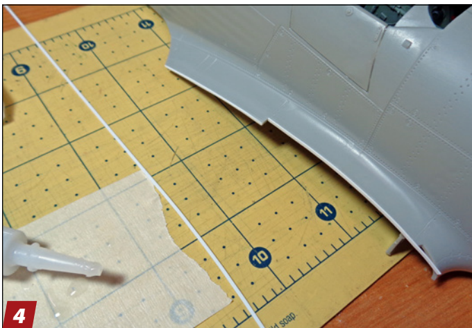
4 Although the subassemblies fit together well overall, a gap between the right wing and wing root required filling. I added a length of thin styrene strip attached with superglue to do the job.
