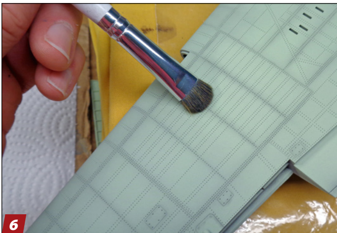
6 Second, I employ a thick, flat makeup brush to remove much of the pastel and blend and soften the effect. Notice, it's not nearly as stark as it was in Step 5, but the dark gray accent remains noticeable.
