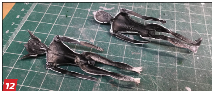
12 After the epoxy set, I drilled holes for the Martian's eyes through the epoxy putty. Then I sprayed the inside of the figure with gray primer, waited for it to dry, and followed up with a coat of black primer. This would help block any potential light leakage.
