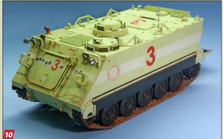
10 After drilling out the headlights, I painted the housings with Alclad II Chrome (No. ALC107) and dropped in M.V. Products lenses. For the lights that point to the sides, I mounted the kit parts on scrap PE bent to make a channel; the light cable is 32-gauge black wire. The lenses for the armored vision blocks and black taillights were finished with decal paper painted with Alclad II Jet Exhaust (No. ALC113), the top-coated with Tamiya Smoke (No. X-19). For the red taillights, I painted decal paper Alclad II Aluminium and Tamiya Clear Red (No. X-27).
