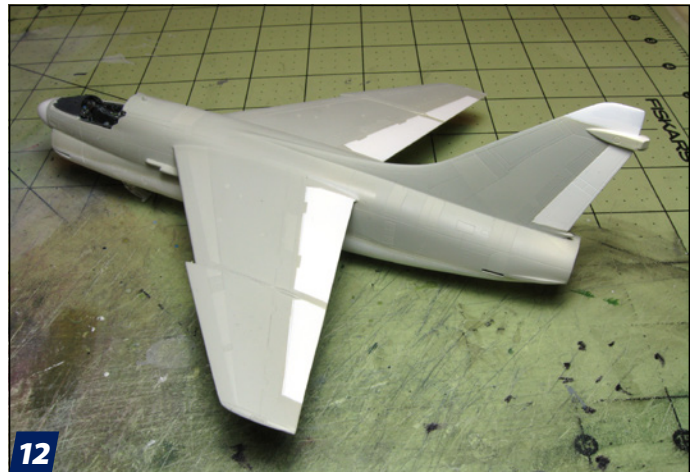
12 To break up the gray, I masked several panels and airbrushed them with light gull gray lightened with a few drops of white. Note the lighter panels on the vertical tail, the segmented panels behind the leading-edge slats, and on the fuselage.
