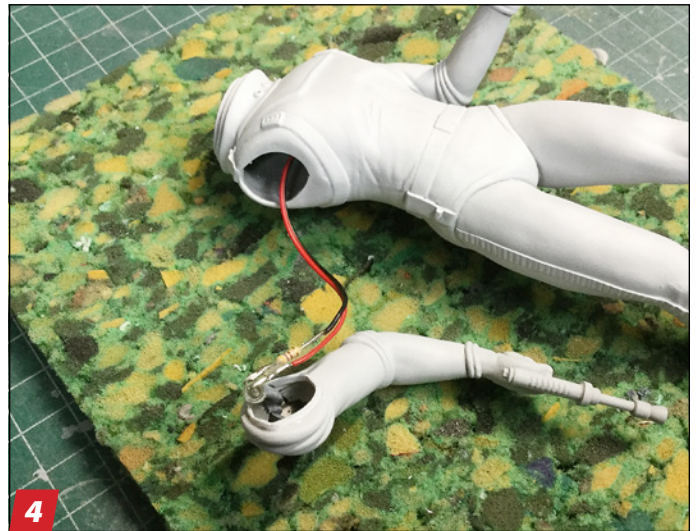
4 I assembled most of Flash's body and ran wires through the torso and one leg to the arm. I mounted the LED to the shoulder, attached the fiber optic to the LED, and soldered the electrical leads and 417 OHM resistor in place.
