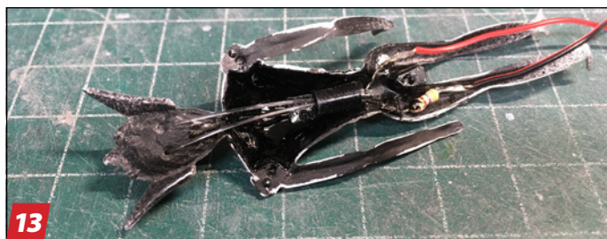
13 I cemented a socket made from Evergreen tube inside the figure cavity. The fibers run through the eye holes and into the open end of the tube. I epoxied a 3mm LED at the other end of the tube with a 417 Ohm resistor and electrical wires running through the legs.
