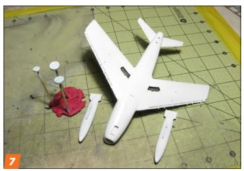
A coat of Testors Gloss White (No. 1145TT) enamel covers the underside of the airplane, the wing tanks, and wheel rims. The main wheel wells were airbrushed a custom mixed dark green and I hand-painted details. I waited until later to paint the nose gear bay.
