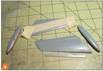
To make the recessed slat housings, I sawed a shallow cut along the rear and ends of the scribed slats. I deepened the cuts with a tapered file and then ran a sanding stick along the leading edges until the entire area matched the depth of the surrounding cuts.
