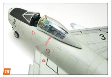
I attached the turtledeck, canopy, windshield, and completed wing slats. A small gunsight made from pieces of plastic was glued to the back edge of the cockpit coaming. I added short black decal strips on the slat housings to represent slat tracks.
