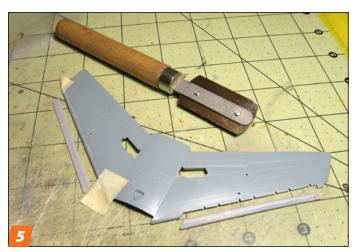
A razor saw proved handy to make notches in the lower portion of the leading edges for slat actuators made from plastic strip. I kept the replacement slats nearby for reference.
