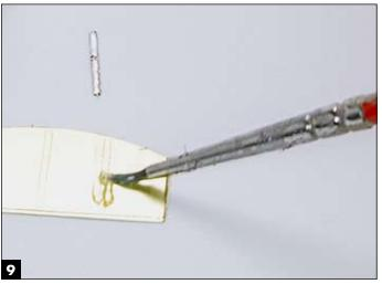
... then paints flux onto the larger part where the rib will attach.
