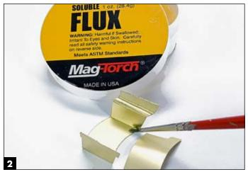
Rick paints flux along the mating edges of Aber's Panzer IV turret stowage bin. Precise flux placement keeps solder where it belongs and minimizes cleanup.
