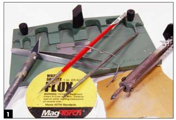
Tools of the trade: Rick's soldering arsenal includes a 40-watt soldering iron, solder, and flux, as well as sandpaper, files, an old paintbrush, a hobby knife, and tweezers. A folding tool, such as Mission Models' Etch Mate, is great for working with photoetched metal.
