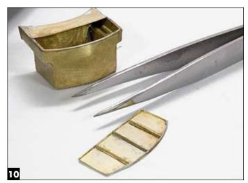
After placing the part, Rick touches the iron to the back side of the detail, melting the solder and binding it to the lid.
