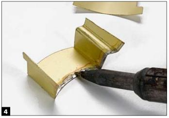
Tinning: Heating the metal part with a soldering iron, Rick melts the solder, then spreads it over the mating surfaces.
