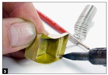
The moment of truth: Holding the tinned parts together, Rick heats the join with the iron, liquefying the solder on both parts and bonding them.
