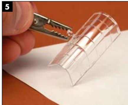
**5** Here's why: No matter how slowly you remove the part, a drop of Future will probably remain at the last point to come out of the bath. If the drop's at a corner, you can drag the corner along a sheet of paper, and the excess Future will wick away. Take a look at the part while it's still wet – if the layer of Future has runs, dust, or looks uneven, simply give the part another dunk in Future and try again. If the coat of Future looks even and smooth, you're ready to let it dry.
