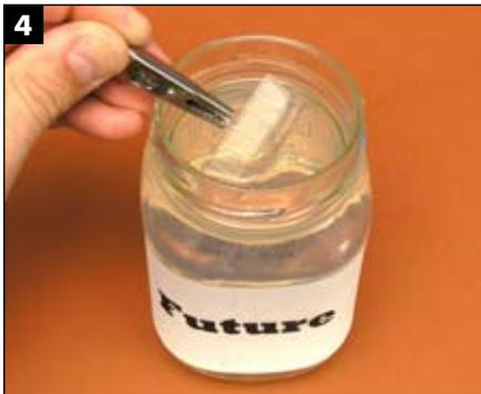
**4** Once the part's thoroughly submerged and you're convinced there aren't any air bubbles, you're ready to remove the part. This is the tricky part. Slowly pull the part out of its Future bath. Removing the part slowly will allow the excess Future to flow back into the bottle and prevent runs. Use the edge of the jar to rest your hand; take your time. When you can, have a corner of the part be the last thing that comes out of the Future.
