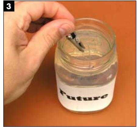
**3** Here's the easy part: Submerge the part in the Future. Just dunk it in. Look for any air bubbles that might be trapped in the part's engraved details. If you see bubbles, turn the part over using the alligator clip and let them float out.
