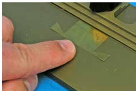
Some photoetched-metal parts must be folded to shape. A bending tool such as this is a big help, especially with larger pieces and longer edges.
