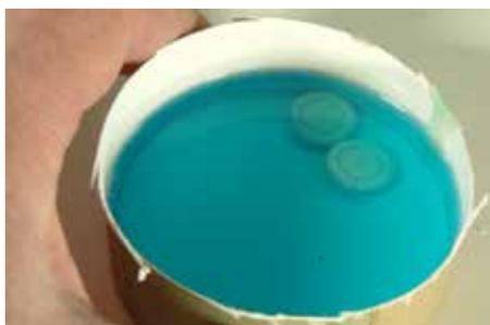
Resin parts, such as these True Detail aircraft wheels, need extra attention to clean off manufacturing residue. Bleche-Wite tire cleaner does the job well, but be sure to wear hand and eye protection — this is strong stuff!
