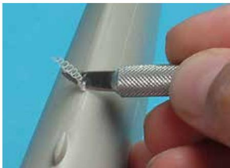
Liquid styrene cement joins pieces by melting the plastic. With judicious clamping, a little plastic will seep out of the joint and close the gap; slicing the excess off cuts down on sanding time.
