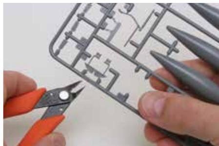
**We've said it before and we'll say it again: Clip, don't twist, the parts from the sprue. A straight-edge razor can help with parts that are hard to reach with clippers.**
