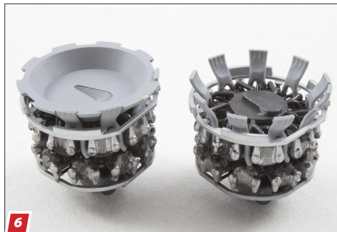
6 ICM included a brilliant jig that makes placing the individual exhaust stacks at the correct angle and orientation a snap. The jig is in place on the left engine along with a handful of stacks; the completed engine on the right shows the stacks with the correct buck-toothed appearance.
