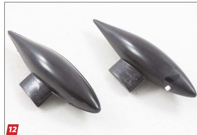
12 The Invader I was modeling, and many other Korean War B-26s, was armed with napalm tanks, which were usually modified large drop tanks. But, the ICM kit includes the smaller, 75-gallon tanks. Luckily, I had a spare set of the large tanks left from a Monogram P-61. The simple modifications seen on the right include removing the centerline stiffening ridge and adding a filler spout made from styrene rod.
