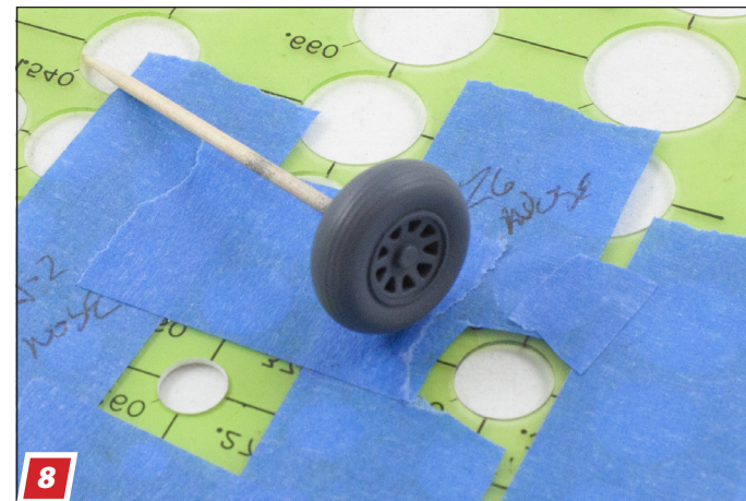
8 I always look for quick ways to mask. Here, I used a circle template to mask the tire while I paint the hub. Simply select the appropriately sized circle and surround it with tape to prevent overspray...
