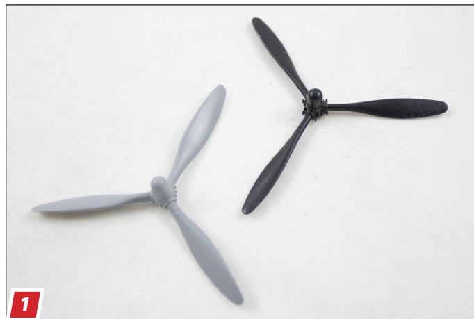
1 One of the simplest ways to improve ICM's B-26 is to swap the props as the kit parts are too plump and the hub lacks detail (left). The props in Monogram kit look much better and I happened to have one of them in my stash.
