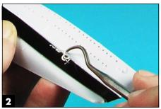
Ted carefully runs a scribing tool along the hull, using the labeling tape as a guide. He makes several passes to cut a deep groove.
