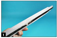
On some models, the waterline is marked with a raised line on the hull. Ultimately, it is up to you to decide how high or low you want your ship to sit in the water. Once satisfied with the waterline location, mark it with plastic labeling tape.
