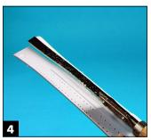
Starting at the bow and working toward the stern, Ted cuts along the groove with a razor saw. "If you find the cutting difficult or the saw binds, go back to the scribing tool and cut a little deeper," Ted says.
