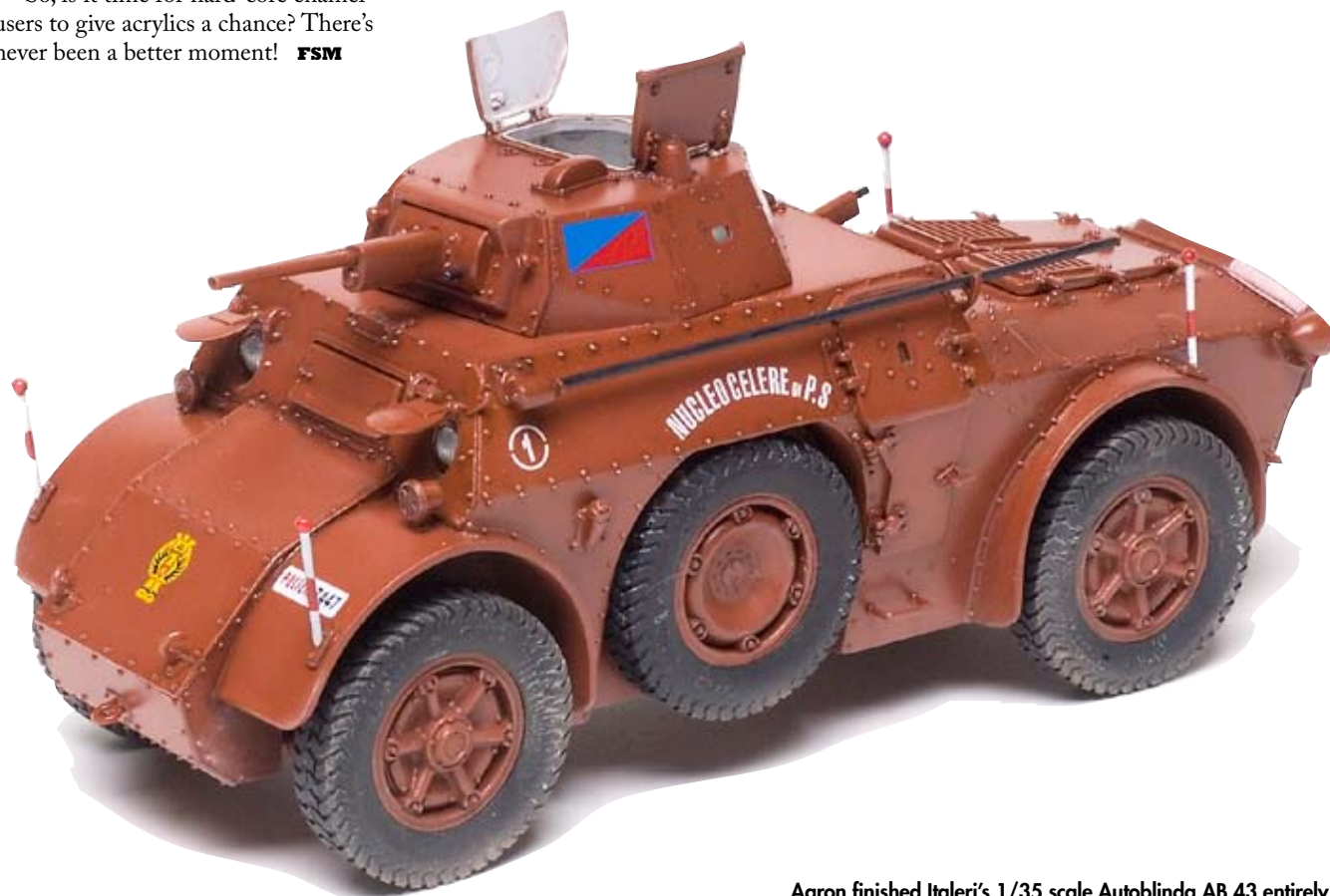
Aaron finished Italeri's 1/35 scale Autoblinda AB 43 entirely with acrylics, including a sludge wash, to model a glossy post-World War II Italian police vehicle.
