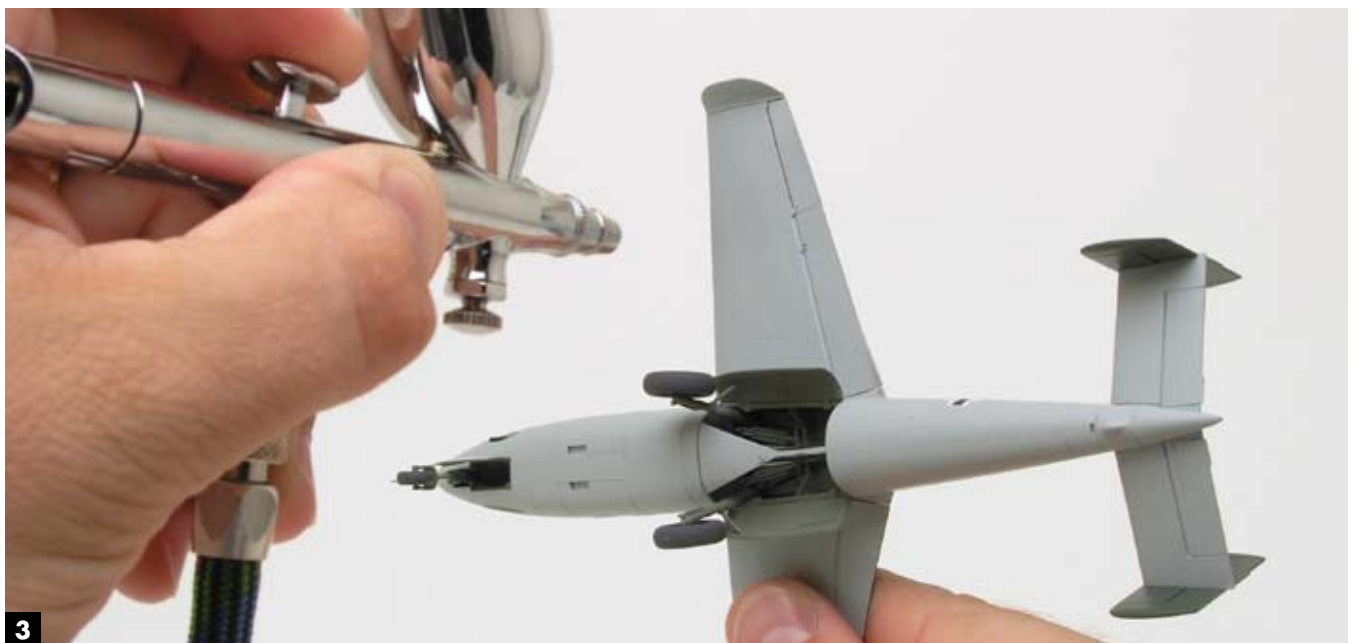
2 The He 162's wing is painted with flat light blue paint. It needs to have a clear gloss coat applied to it before the insignia decals go on.
