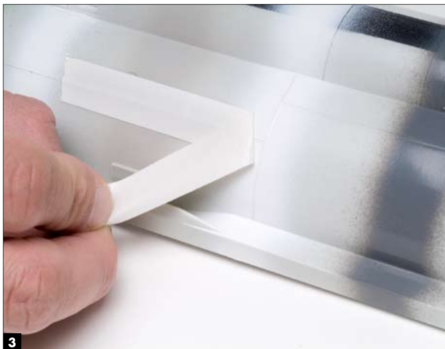
Aaron peels Scotch Paper Tape away from a sample to test the paint's durability and adherence.
