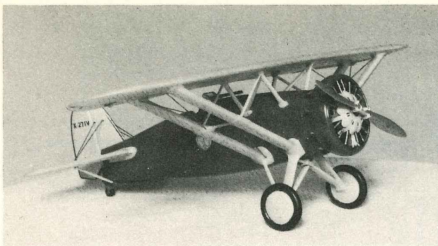
The Army's XP-15, X-270V, was externally identical to the XF5B-1 except for the absence of an arrestor hook, so Ned used a photo of the Army plane when modeling details on the right
