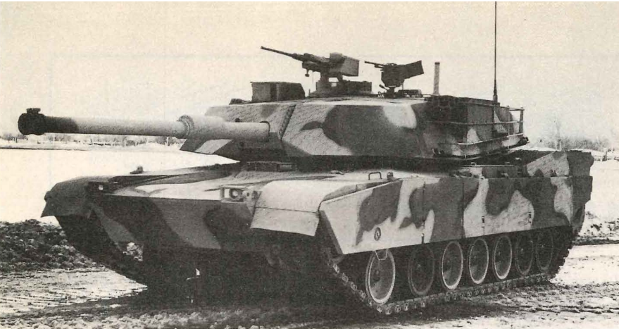
(Above, below, and bottom) The XM1 prototype, unveiled at Warren, Michigan on February 3, 1978, differed from the production version shown in the drawings in several details. This is the "snow-open terrain" camouflage scheme.
