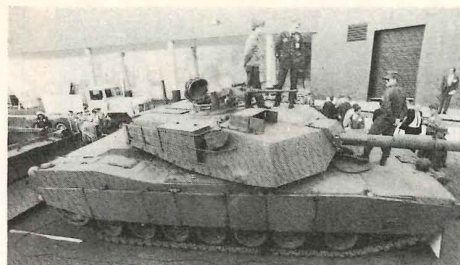
This production M1 clearly shows the commander's station on the turret roof, the large flash suppressor over the coaxial machine gun, and the prominent hull skirts.
