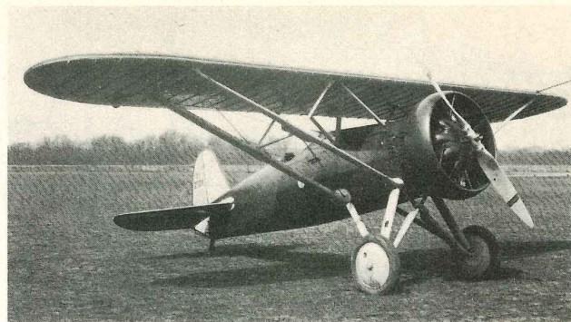
side of the fuselage. Note the unusual structure of the forward landing gear, the triangular brace inside the cowling, and the wires supporting the vertical and horizontal stabilizers.
