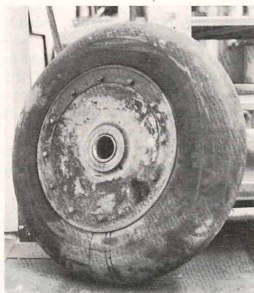
(Above left) FIG. 4. The propeller spinner before restoration. Colors are a white spiral over an azure base. (Above right) FIG. 5. One of the main landing gear wheel and tire assemblies. The solid cast wheel is painted semigloss black. American technicians probably applied these colors to the spinner and wheel after the war.
