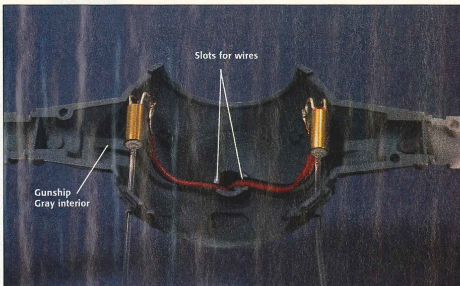
9 The lighting system in place before installation of the cockpit assembly. Trim the fiber-optic strands to the correct length before gluing them in place.
