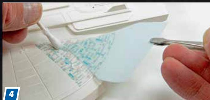
4 Once the decal moves freely on the backing paper, I placed it on the model and slide the paper out while holding the decal in position with a cotton swab. Avoid using your finger on the decal as it will often stick to skin. Use the swab to carefully refine the position of the decal.
