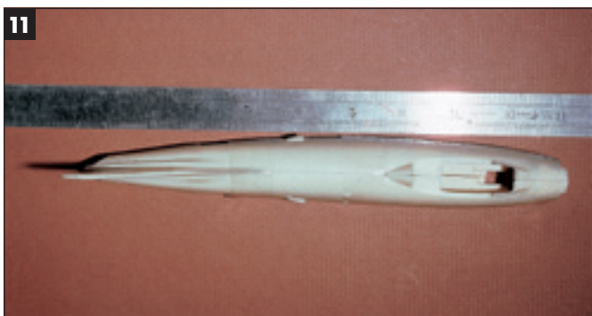
11 Warpage can be a problem with resin castings such as these F-86H fuselage halves.
