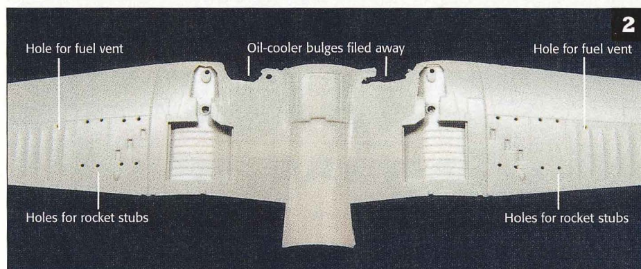
Holes for rocket stubs and fuel vents are drilled in the wing.
