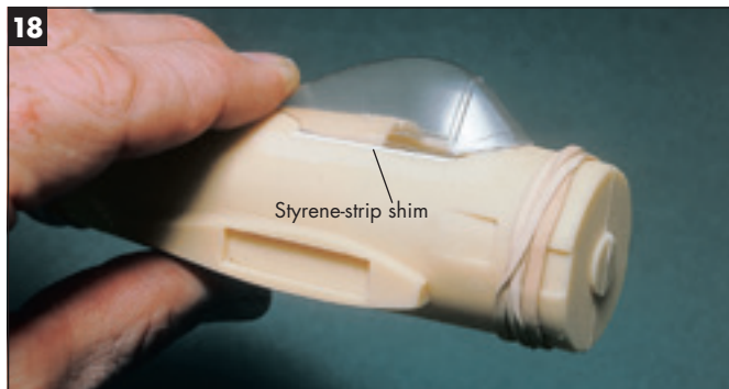
18 Pat filled gaps around the Fireball canopy with styrene strips.
