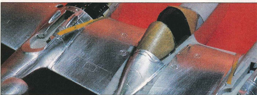
10 With the foil burnished in place, the edges can be trimmed with a sharp blade.
