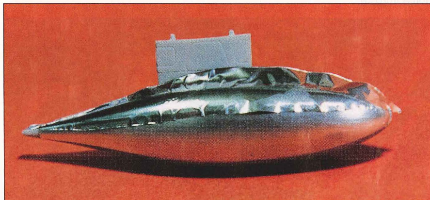
4 The next piece of foil overlaps the first and then is burnished in place.
