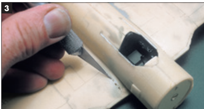
3 Larger surface bubbles must be “drilled out” like a cavity in a tooth in order for them to hold filler material.
