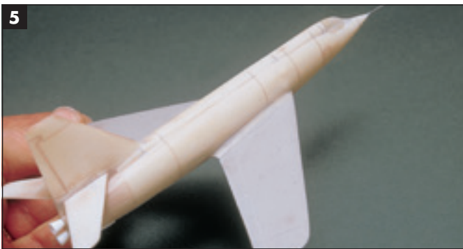
After scribing in control surfaces, the new wing looks as good as . . . new!
