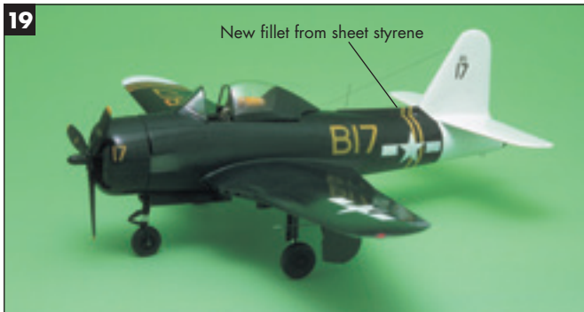
This hybrid (reciprocating and jet engines) FR-1 Fireball was made from the out-of-production 1/48 scale Nero kit.
