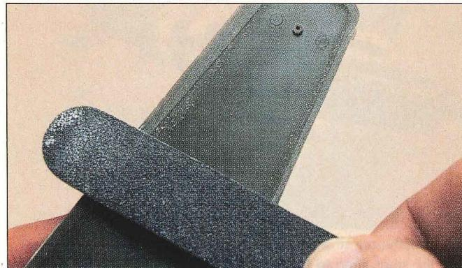
**5** Since sanding seams would mean saying goodbye to the factory finish, it was important to strive for as precise a fit as possible. Here the inner surfaces of the wings are smoothed of any raised blemishes with a coarse sanding stick.
