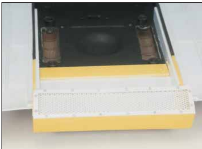
8 Extruded-aluminum mesh has the correct diamond-shaped pattern for the exhaust grille.
