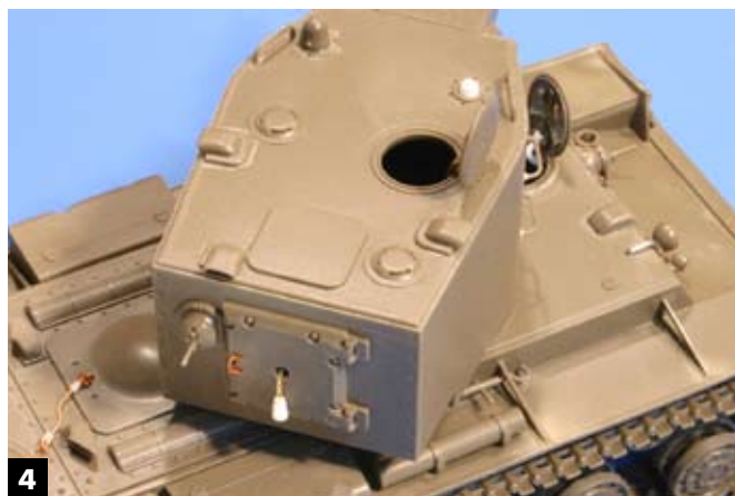
4 After drilling out a pistol port, Charlie chucked a chunk of styrene into his motor tool to make a plug he attached to a bit of leftover chain.
