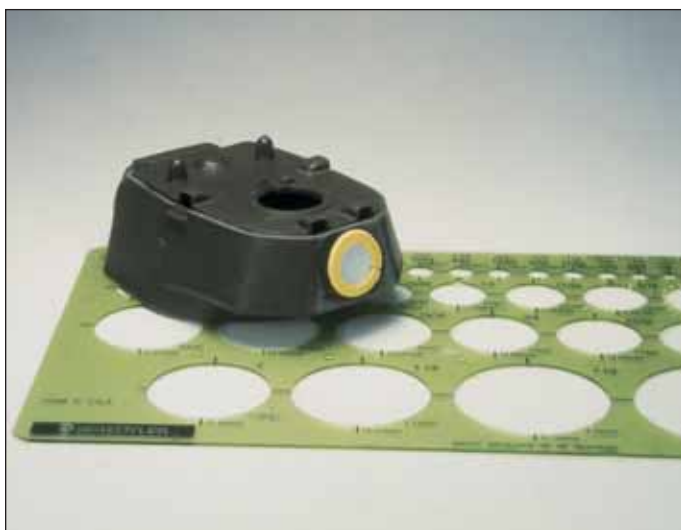
13 A circle template helped make a reinforcing ring for the rear machine-gun mount.
