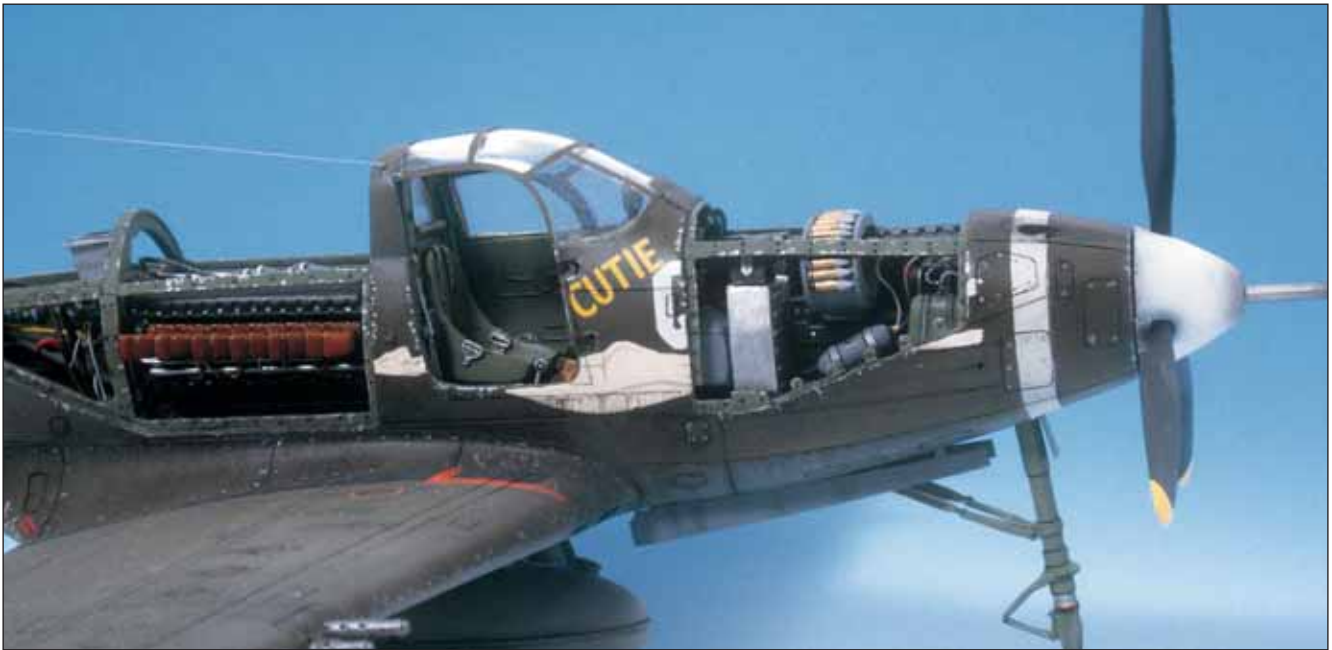
With the engine cover, cockpit doors, and gun bay covers removed, the model depicts an aircraft under maintenance.
