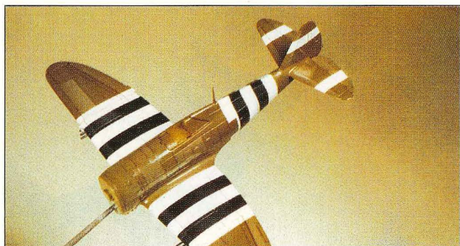
16 The clear gloss overaccentuates the shaded panels. The oil wash deepens the panel lines.
