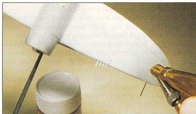
7 Light, dusty coats of acrylic establish "teeth" for heavier color coats to come.
