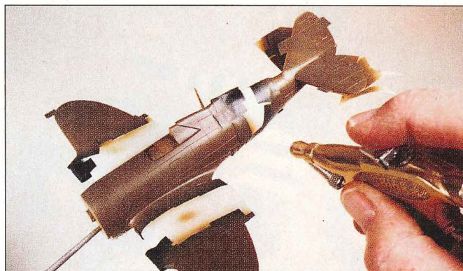
10 To achieve sharp lines, Walt sprays at 90 degrees to masked color demarcations.
