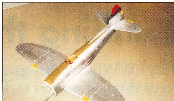
19 Various shades of Alclad were used to differentiate panels. The masks have been removed from the pre-painted areas.
