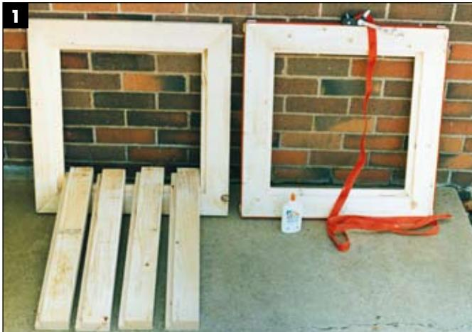
**On the lower left are four frame pieces, each with a dado to hold a sheet of plywood; the beveled cuts at the end of each piece (seen in the assembled frames leaning against the wall) are still to come. The frame on the right shows a Pony band clamp in place with the ratchet tightener at the top of the frame.**
