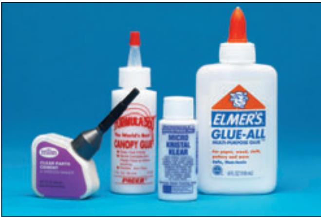
Some parts, such as clear canopies, windshields and chrome-plated trim, don't react well to standard modeling glues. Testor's Clear Parts Cement, Microscale Micro Kristal Klear, Pacer Formula 560, and even Elmer's Glue-All white glue are great choices for installing clear parts. These glues can be thinned with water and flowed into joints with a fine-point paintbrush, 1. They're stronger than you might think, and they're non-toxic, too, so they're good choices for young modelers.
