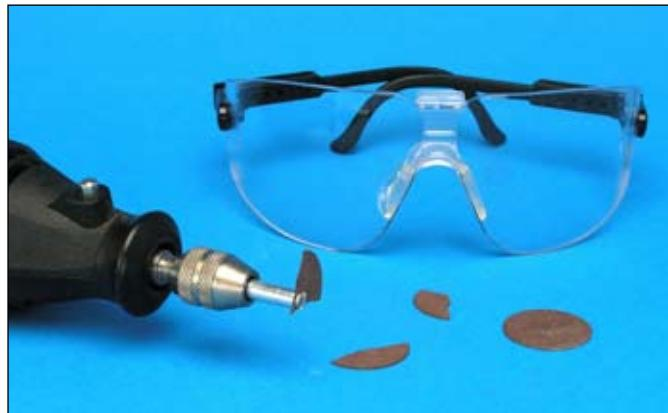
When you use a motor tool or most of the cutters outlined here, it's always a good idea to wear a good pair of safety goggles, which are available inexpensively at hardware and home stores. Cutting wheels can break, and tiny bits of wire and plastic can go flying — protect yourself properly.
