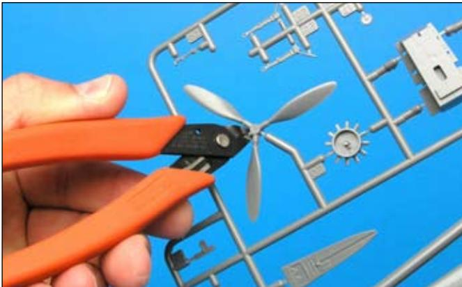
Cutting shears are a great all-purpose tool, but they're especially handy for removing delicate parts from the sprue. This pair is from Xuron ([www.xuron.com](http://www.xuron.com)). Precision shears like these save lots of time at the workbench. What little sprue remains on the parts can be trimmed away with a hobby knife.
