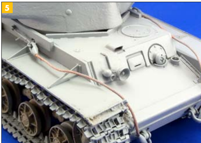
5 This time, Mike applies a smooth coat of Mr. Surfacer 500 for primer.
