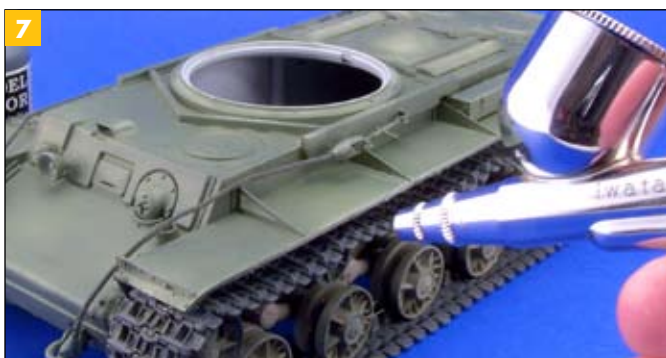
7 White-metal tracks were primed, then airbrushed with a base coat of Vallejo Model Color black grey.
